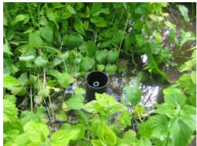
Borehole SU98SW110 and close-up showing the observation tube within the outer casing.
