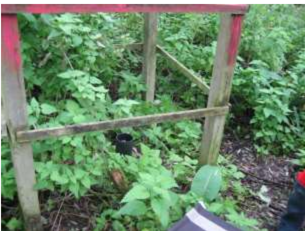
Borehole SU98SW110 and close-up showing the observation tube within the outer casing.
