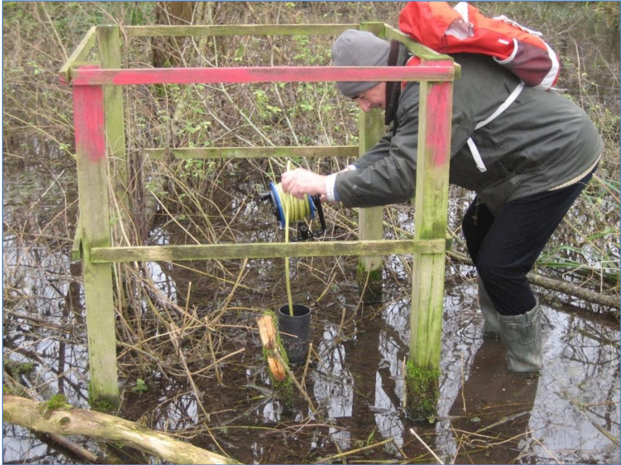
Borehole containing a tube-well in the willow fields. Ian Caird (Maidenhead Waterways) measuring groundwater depth using an electronic dip sensor.
